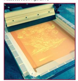
Figure A. Here, 20" x 24" OD static aluminum frames stretched to 20 N/cn were used to print the sea turtle. A 156-mesh was used for the white underbase and 230-mesh for the colors. Notice the amount of detail in the white underbase print. - See more at: http://impressions.issshows.com/screen-printing-designs/Screen-Printing-on-Fleece-8356. shtml#2
