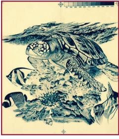
Figure B. Notice the grey scale in the top right-hand corner of the film positive. Exposing this grey scale on each screen for every color is a great way to visually inspect that all the halftone dots from the 5%-100% tonal range are exposed and washed out properly - See more at: http://impressions.issshows.com/
