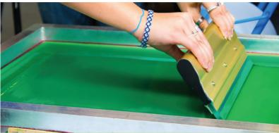
If the imprint cracks when flexed or stretched, improper curing is the likely problem. In cases where too much mineral spirits or non-curable reducers are added for thinning, the plastisol ink will not fuse no matter how long or how hot the cure.
