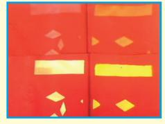
White Discharge......Color Discharge. Fixation through Pressure Steaming 2.5Bar for 30Min.
